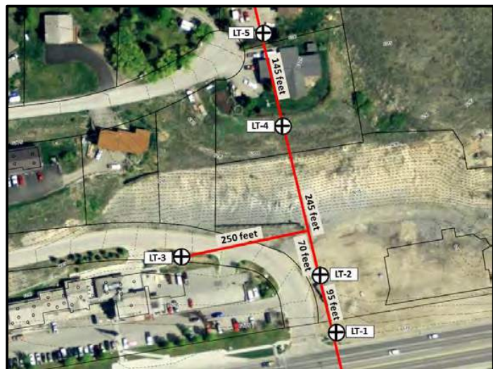
Figure 9: Location of drill holes LT-1, 2, 3, 4, 5, and the nearly north-south cross section (solid red line) on an air photo taken in 2013. Lot and parcel lines are shown in black including an outline of the Walgreens store completed in late 2013.
