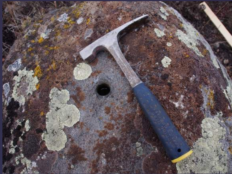
Turpin Meadows USGS Benchmark 1 st elevation established in Jackson Hole by differential leveling.
